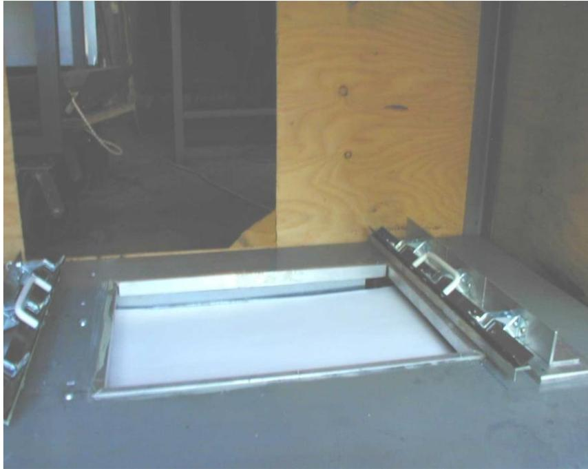
*Figure B-7. Paper Tray Below Welding Pad or Blanket – Paper Ignition Test.*
